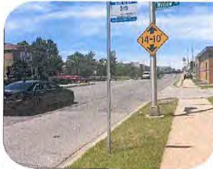
This transit stop lacks any dedicated space for passengers to board or disembark from the bus.
